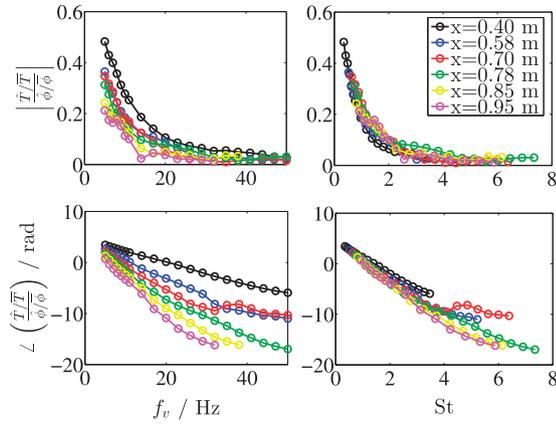
**Figure 7.** Absolute value (top row) and phase (bottom row) of the transfer function between the normalized temperature fluctuations and the normalized equivalence ratio fluctuations for  $\dot{m} = 180$  kg/h; plotted over frequency (left column) and the Strouhal number (right column).
