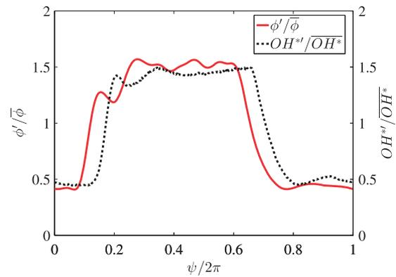
**Figure 4.** Relative fluctuations of the equivalence ratio and the  $\text{OH}^*$ -intensity over one period of fuel modulation at  $f_v = 20$  Hz.
