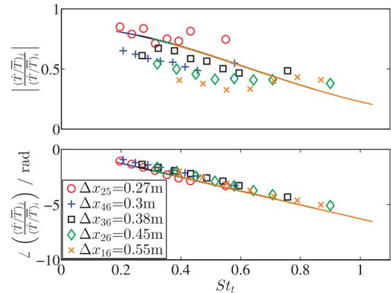
**Figure 11.** Absolute value (top) and phase (bottom) of the measured (marker) and modeled (line) transport transfer function  $\hat{H}_t$  for different convection lengths  $\Delta x_{ij}$  (colors) and an air mass flow of  $\dot{m} = 220$  kg/h;  $Pe = 30$ .
