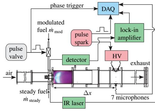
**Figure 3.** Schematic of the combustion chamber setup.
