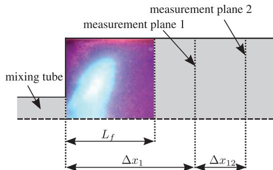
**Figure 9.** Display of model parameters and measurement planes.
