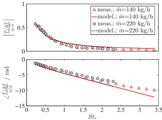
**Figure 10.** Absolute value (top) and phase (bottom) of the measured (solid) and modeled (dashed) reactor transfer function  $\hat{H}_t$  for different mass flows  $\dot{m} = 140$  kg/h (red) and  $\dot{m} = 220$  kg/h (black);  $\tau_r = 55$  ms;  $\Delta x = 0.4$  m.
