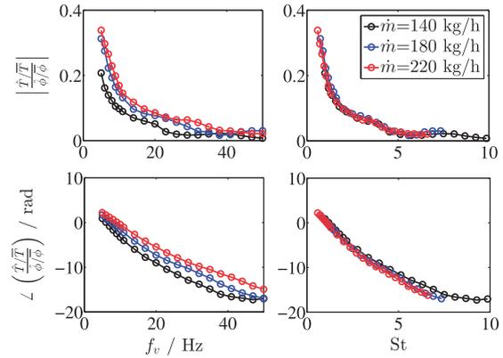
**Figure 6.** Absolute value (top row) and phase (bottom row) of the transfer function between the normalized temperature fluctuations and the normalized equivalence ratio fluctuations at  $\Delta x = 0.78 \text{ m}$ ; plotted over frequency (left column) and the Strouhal number (right column).
