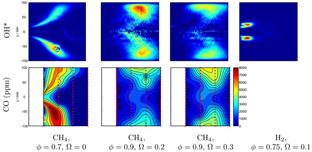
Figure 3: Abel deconvoluted  $\text{OH}^*$  chemiluminescence and local gas concentrations for the premixed combustion system. Adiabatic flame temperatures between 1560 K and 1600 K. (Injector outlet on the left side. Measurement locations indicated by red crosses.)
