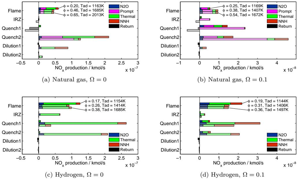
Figure 10:  $\text{NO}_x$  production in different reaction network zones of RQL combustor ( $T_{in} = 650 \text{ K}$ ).
