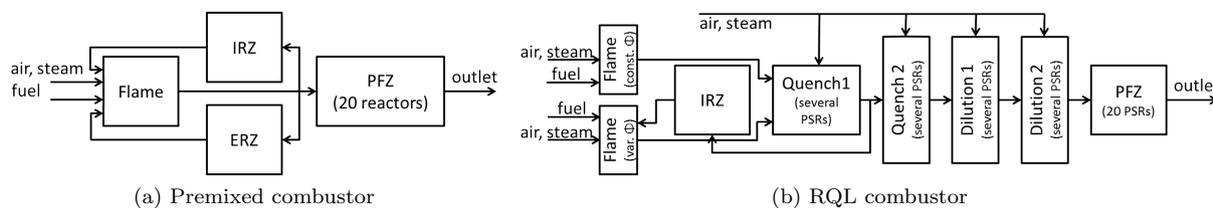
Figure 2: Chemical reactor networks.
