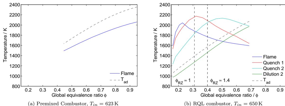
Figure 6: Average temperatures of the reactor network zones for operation with natural gas at dry conditions.
