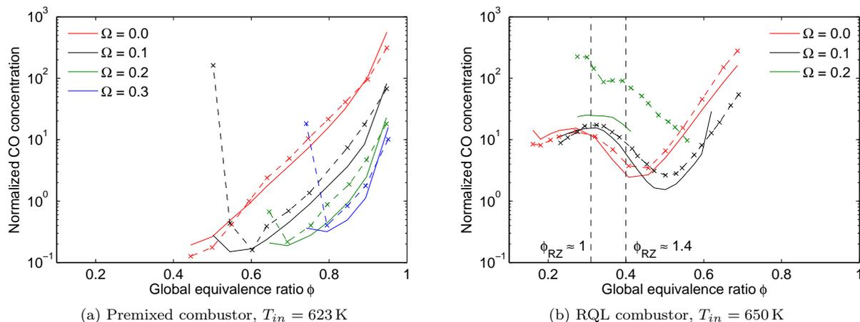
Figure 5: CO emissions for natural gas. Experimental data ( $-x-$ ) and simulation results ( $-$ ). Data normalized with the value of the premixed combustor at  $\phi = 0.6$ ,  $\Omega = 0$ .
