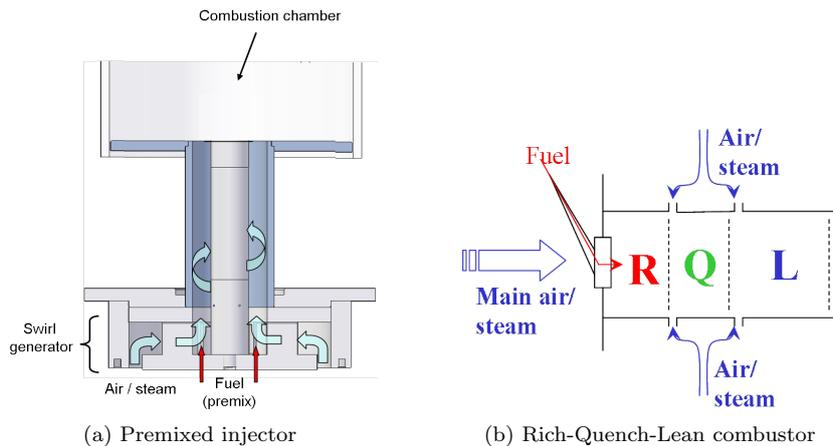
Figure 1: Combustion systems.
