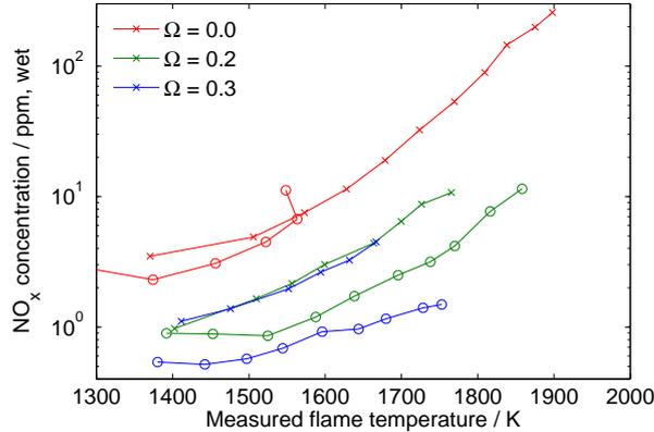
Figure 8: Measured  $\text{NO}_x$  concentration and flame temperature in the premixed combustor [9]. Operation with natural gas ( $\text{---}\times\text{---}$ ) and hydrogen ( $\text{---}\circ\text{---}$ ). The equivalence ratio was decreased from  $\phi = 0.95$  (dry  $\text{H}_2$  flame from  $\phi = 0.55$ ) to blowout for each curve.
