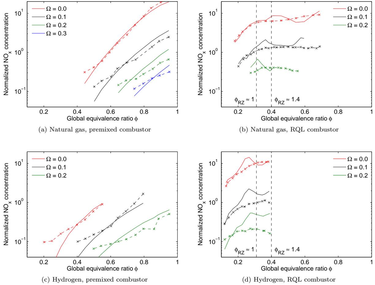
Figure 7:  $\text{NO}_x$  emissions for natural gas and hydrogen. Experimental data ( $-x-$ ) and simulation results ( $-$ ). Data normalized with the value of the premixed combustor at  $\phi = 0.6$ ,  $\Omega = 0$ .
