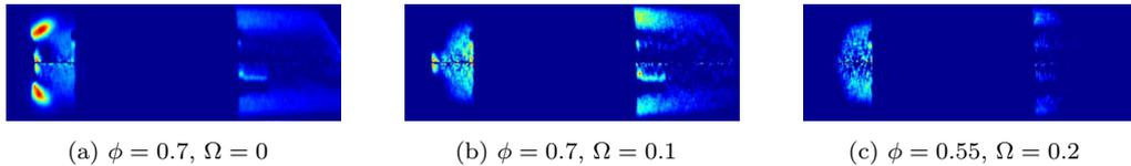
Figure 4: Abel deconvoluted  $\text{OH}^*$  chemiluminescence images of the RQL combustor. Rich zone is on the left, dilution zone on the right, the quenching zone is hidden by the injection manifold. (NG,  $T_{in} = 650$  K)
